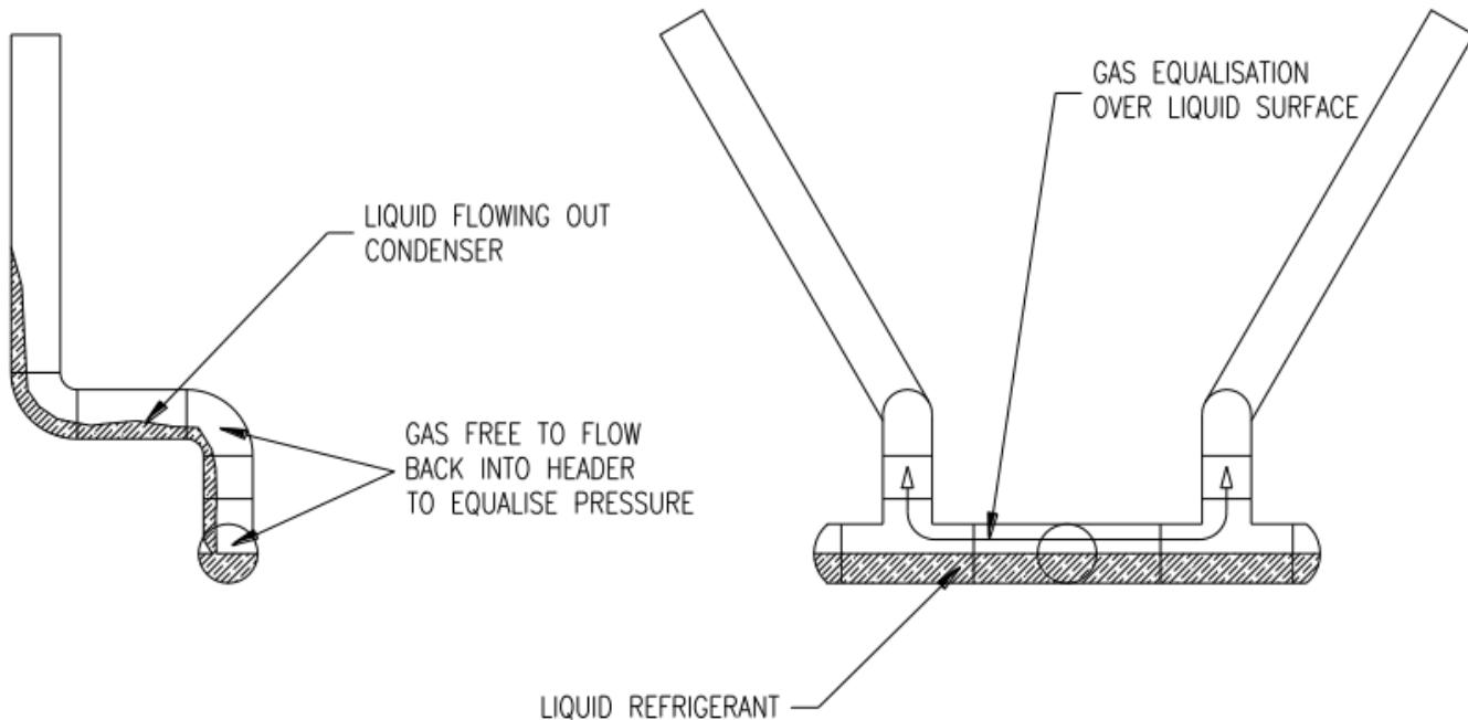
When piping up to a twin coil condenser it is most important to observe the above principal. A lack of good drainage will cause liquid to back up in the condenser coil giving substantial reduction in capacity.
