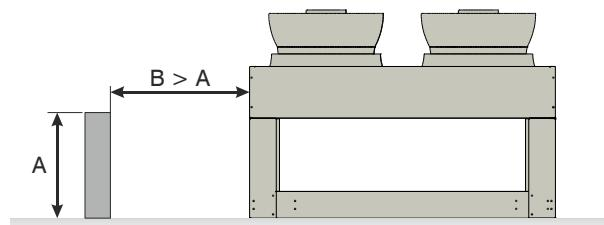
2.1.2 Parapet walls near the unit:
