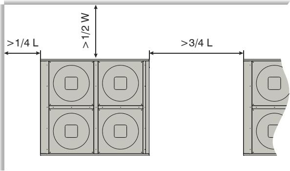
2.1.6 Installation with walls on 3 sides, (1 side fully open):
